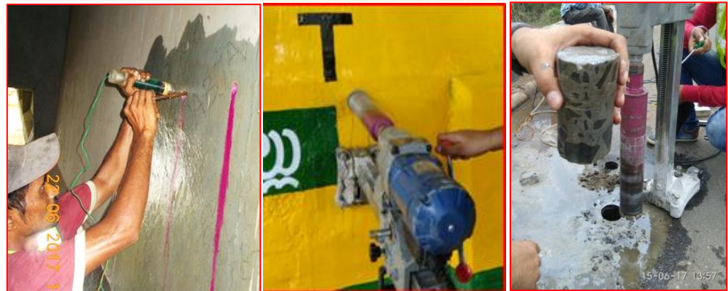
Carbonation Depth Test and Core Cutting
